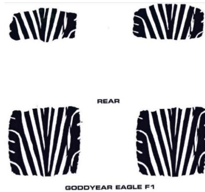
Figure 2.10: Vehicle at Acceleration Tire Patches
