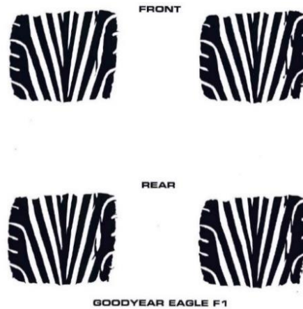
Figure 2.9: Vehicle at Rest Tire Patches
