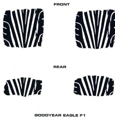
Figure 2.11: Vehicle at Deceleration Tire Patches
