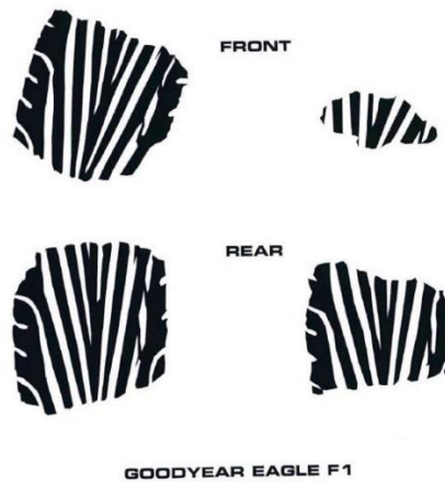
Figure 2.12: Vehicle at Turn Tire Patches
